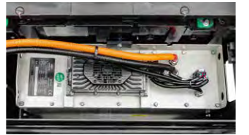
(Option) Lithium battery with the on-board charger (48V, 20A) (Excluding model F2)
